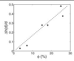
FIG. 4.  $\Delta h(d)/d$  as a function of porosity  $\phi$ . Range of bead diameters used to realize samples: 104–128  $\mu$ m ( $\Delta$ ): dynamic fracture, ( $\square$ ): quasistatic fracture; 50–65  $\mu$ m ( $\diamondsuit$ ): dynamic fracture. The slope of the dashed line is 1.7.
