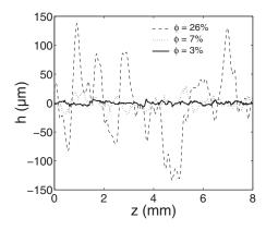
FIG. 1. Height profiles extracted from fracture surfaces of three sintered glasses with three different porosities but with beads with the same diameter 104– $128~\mu m$ .
