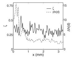
FIG. 3. Variations of the roughness exponent  $\zeta$  and amplitude  $\Delta h(d)$  with the distance x to the initiation notch for the same sample ( $\phi = 3\%$ ) as in Fig. 2.
